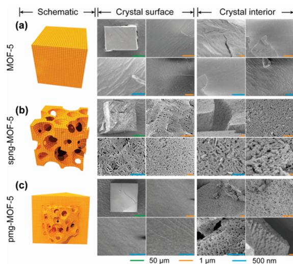
**Figure 2.** Pore structures of MOF-5, spng-MOF-5, and pmg-MOF-5 revealed by SEM observation of their crystal surface and interior (scale bars, green 50  $\mu\text{m}$ , red 1  $\mu\text{m}$ , blue 500 nm).
