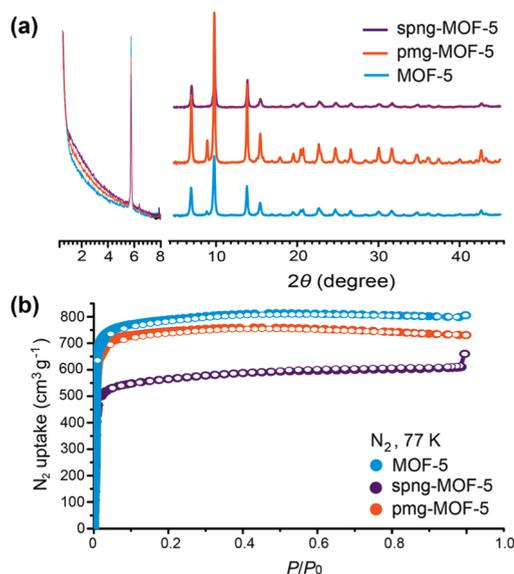
**Figure 1.** Typical analysis performed on MOF-5, spng-MOF-5, and pmg-MOF-5. (a) X-ray data of crystalline powder of MOF-5, spng-MOF-5, and pmg-MOF-5, (b)  $\text{N}_2$  adsorption isotherm at 77 K with adsorption (●) and desorption points (○).  $P/P_0$ , relative pressure.
