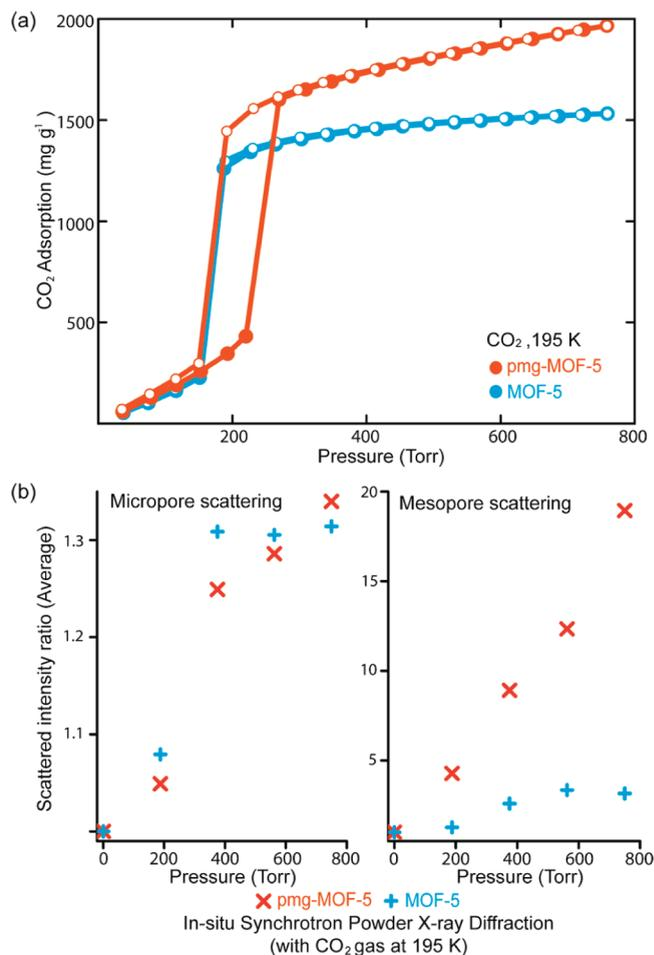
**Figure 4.**  $\text{CO}_2$  adsorptive properties for pmg-MOF-5 and MOF-5. (a)  $\text{CO}_2$  uptake at 195 K for pmg-MOF-5 (red) and MOF-5 (blue), adsorption (●) and desorption (○), respectively. Connecting lines are guides for the eyes. (b) In situ synchrotron powder X-ray diffraction as a function of gas pressure for pmg-MOF-5 (red) and MOF-5 (blue). The standard value for scattered intensity ratio is the peak intensity at 0 Torr.
